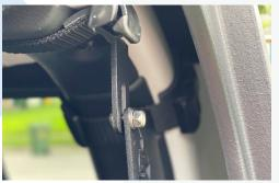
4. Using the supplied bolt, washers, and nut, loosely attach the main panel to the top mount. You can let it hang momentarily. Set up and loosely install the hardware at the bottom bracket as well.
