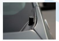
6. Insert a post through the hole with the threaded screw facing down, and ttach via the threaded fender mount from step 2. Hand tighten with a 17mm wrench.
